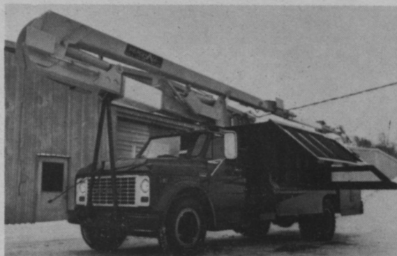
Hydraulically operated chip boxes, either side or end ejection.
