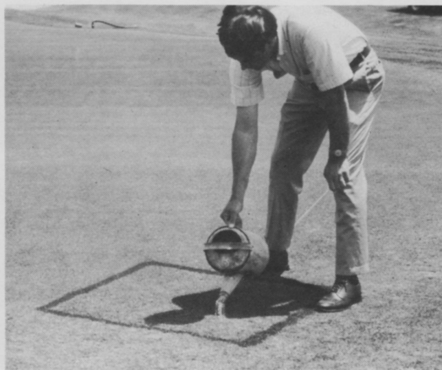
The mixture is applied to one square yard of turf or lawn. Applications should be made on two or three similar areas per 5,000 square feet of turf. Sensitive insects emerge within 10 minutes after application.
