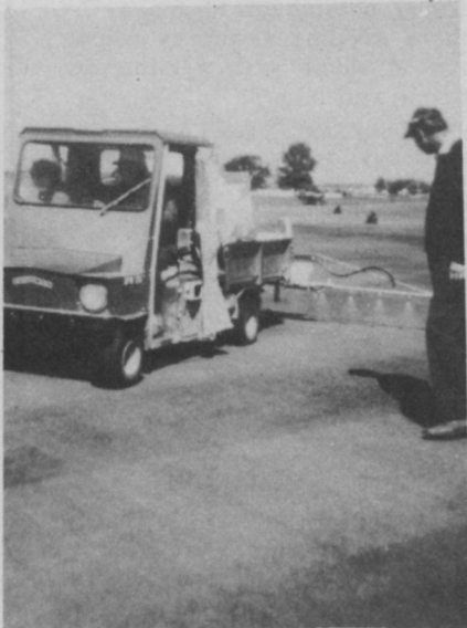
Graf has adapted this truckster to handle a spray rig. It allows him to pull right across greens without any damage.
