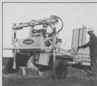
1560 Stump Cutter ... 65 hp unit.
