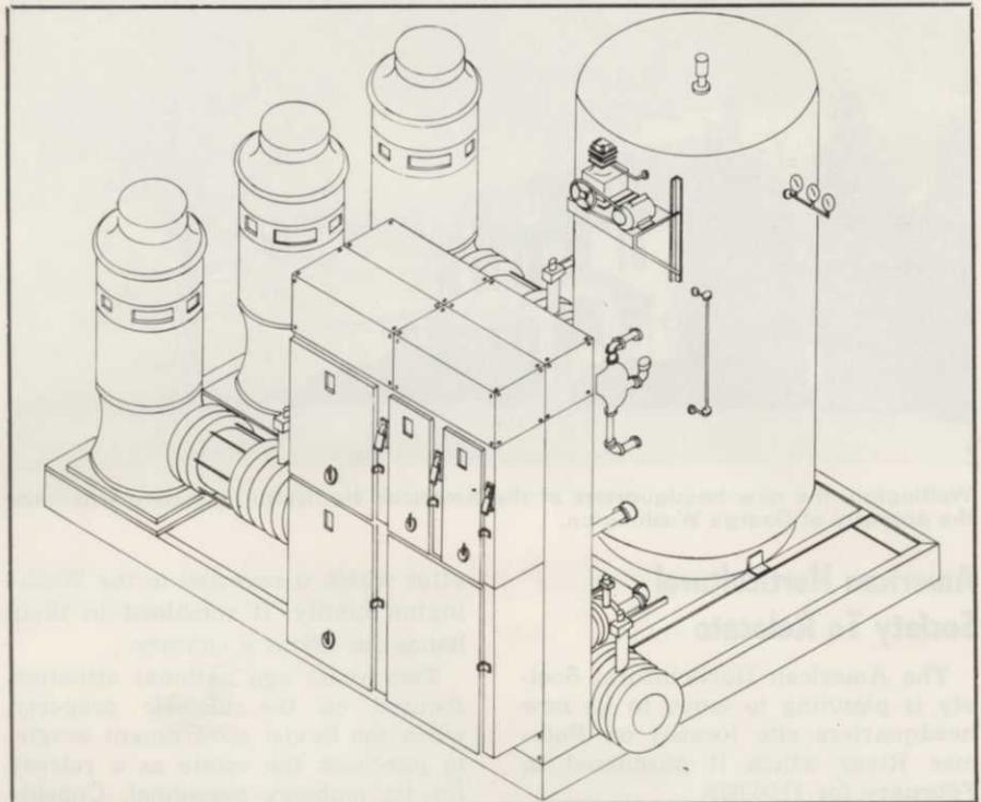
matic, using vertical, centrifugal or turbine pumps. The plant consists of three pumps operating on a demand basis until total output has been reached.
