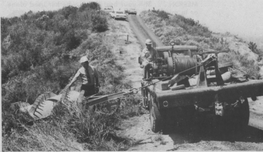
Developer, G. I. Morrow, inspects his invention, a unique brushroller. This picture, taken by the Los Angeles Department of Water and Power, shows that the modified spiked road compactor can pulverize and compress more than 8,000 sq. ft. of hillside brush an hour.
