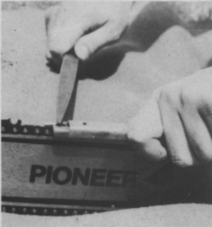
For best cuttings, chain guides should be checked regularly and filed to recommended clearance. (All photos are courtesy of Jeff Dobbs.)
