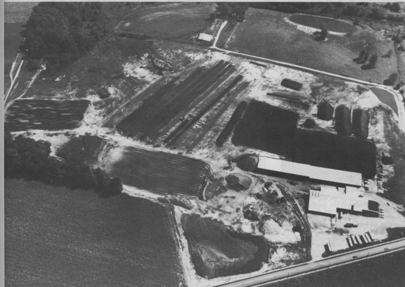
Here's the sixty acre plant of Organic Compost Corporation in Oxford, Pa. The plant takes raw manure that might cause pollution problems, puts it through processing, mixing and composting, and then packages it for sale in a variety of prod-
