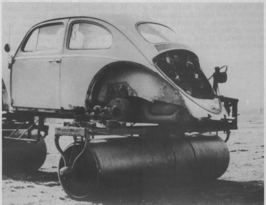
BEETLE ROLLER — a stripped down Volkswagen does yeoman work as a turf roller for Willow Grass Farms, Fort Wayne, Ind. A 3-in. sprocket on rear axles and an 8-in. sprocket on the rear rollers gear the useful rig down to a practical speed. Steering is eased by a power steering pump driven off the fan belt.
