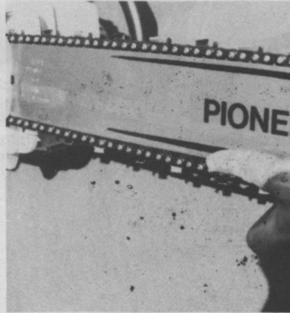
A pull at the bottom of the bar will tell if chain is too loose or tight. (Proper tension shown.)
