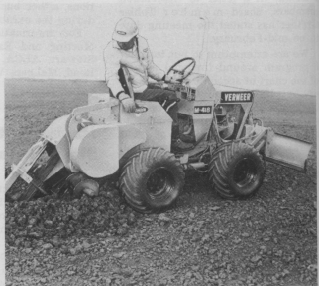
M-418 TRENCHER: Vermeer Manufacturing Co., Pella, Iowa
