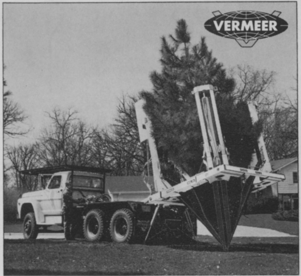
Truck-mounted TS-66T Tree Spade transplants big 6" diameter tree with hydraulically-operated, high tensile steel spades. Digs 66" diameter tree ball, down to 60" deep to prevent root damage.
