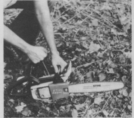
Many accidents occur when first starting saw. Make sure you have a firm grip before pulling starter.
