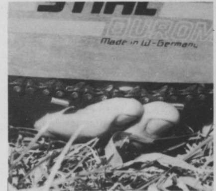
Chain that's too loose can cause saw to "kick back" dangerously. Check chain tension before each use.
