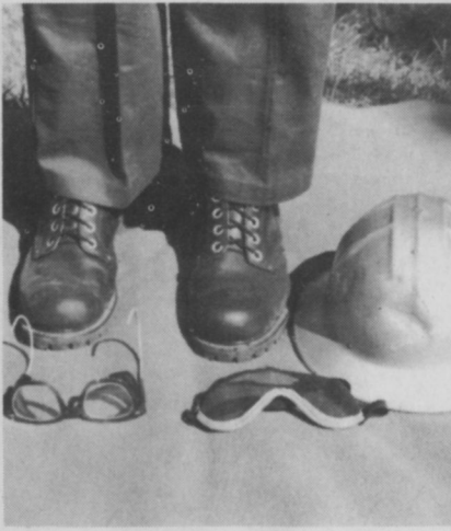
Proper protective clothing is a big part of power saw safety. Note the newer type of screen-style protectors (on right).
