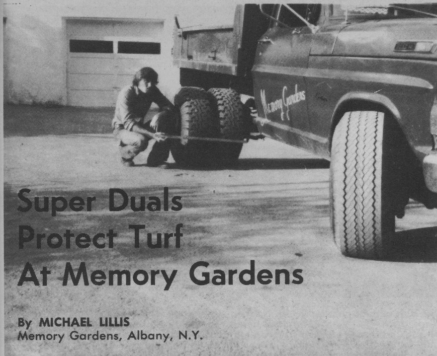
Author (left) measures the width of the super duals. Even when loaded, truck floats over turf. (Above) Ruts tell the before story.
