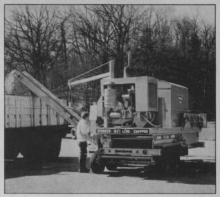
It's automatic! Just load any log or piece of wood-up to 4' wide, 6' long-into the hopper... where carbide-tipped cutting teeth chew it to chips in minutes. Handy conveyor then deposits chips in truck for easy discosal.
