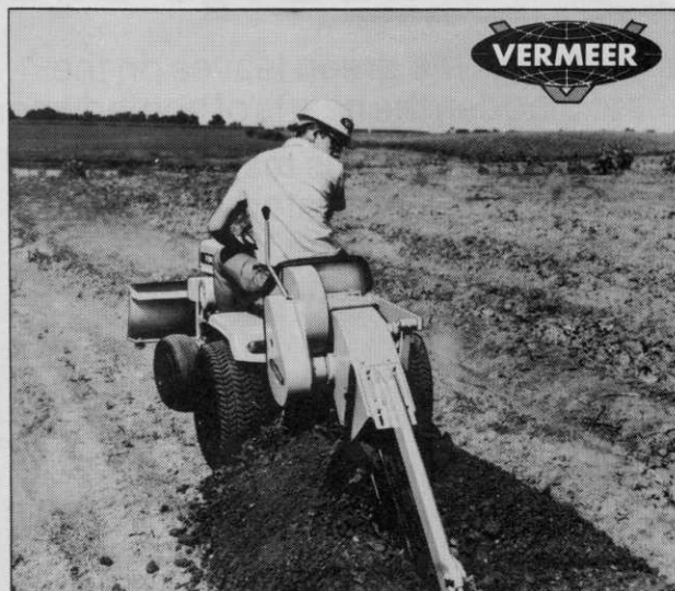
Vermeer M-147H . . . as a mini-trencher, digs 3"-5" wide, down to 30" deep (standard) . . . as a mini-plow, direct buries service lines down to 15" deep . . . as a mini-blade, pushes spoil back into trench with 30° angle, left or right. Available with mini-size trailer.
