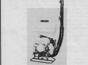
The standard unit is delivered from the factory assembled and ready for spraying. The newly designed solution tank is always completely emptied, making cleaning easy. The engine with blower is mounted on flexible bushings so that no engine vibrations are transmitted to the carrying frame.
