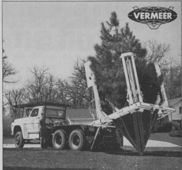
Truck-mounted TS-66T Tree Spade transplants big 6" diameter tree with hydraulically-operated, high tensile steel spades. Digs 66" diameter tree ball, down to 60" deep to prevent root damage.
