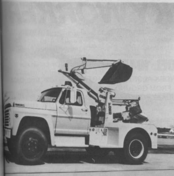
TRUCK-MOUNTED BACKHOE: Tractor and Implement Operations, Ford Motor Company, Troy, Mich.
