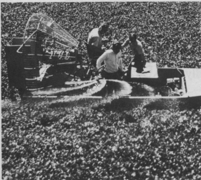
A small motor which operates from the 12-volt battery on the air boat, above, drives the Directa Sprayer unit. Arc of the spray pattern can be adjusted to 90, 180 or 360 degrees.
