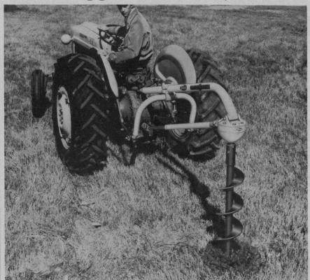
**BUILT RIGHT...PRICED RIGHT!** For agricultural and industrial applications. Two-in-one implement: Rugged post hole digger...or, handy utility crane. Choose from three different size augers: 6, 9, or 12 inch... each 48 inches long. Full swiveling hook (optional) converts unit into 1500 pound capacity utility crane.
