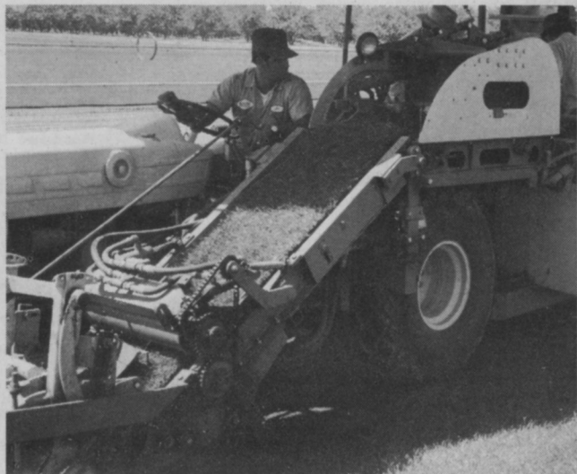
This Nunes sod harvester can cut, lift, roll or slab and palletize more than 1000 square yards of sod per hour.
