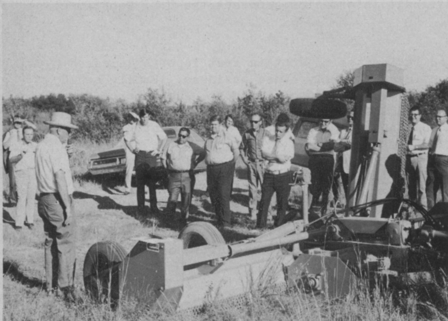
Caldwell Equipment Co.'s version of a flail mower also catches the attention of industrial weed controllers as it is demonstrated and explained. Note the hydraulically controlled wings which can be lifted independently of each other.
