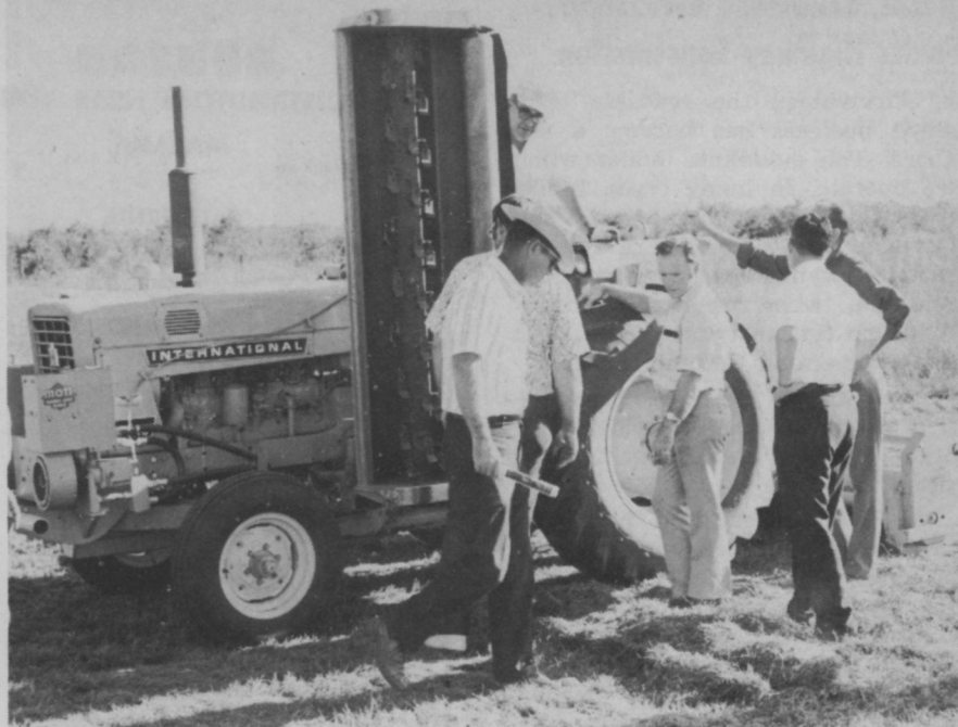
Several industry representatives inspect the cutting job done by this Mott flail mower. Complete hydraulic control makes the mower and tractor easy to operate. This unit has a wing on each side and one in the rear.
