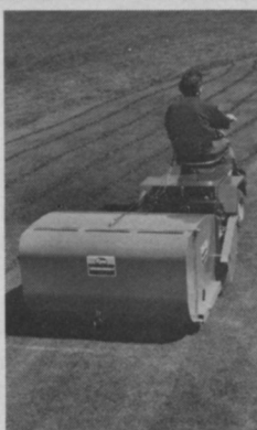
Big, soft 6.50 x 8 turf tires on vehicle and trailer protect turf ... provide smoother ride.
