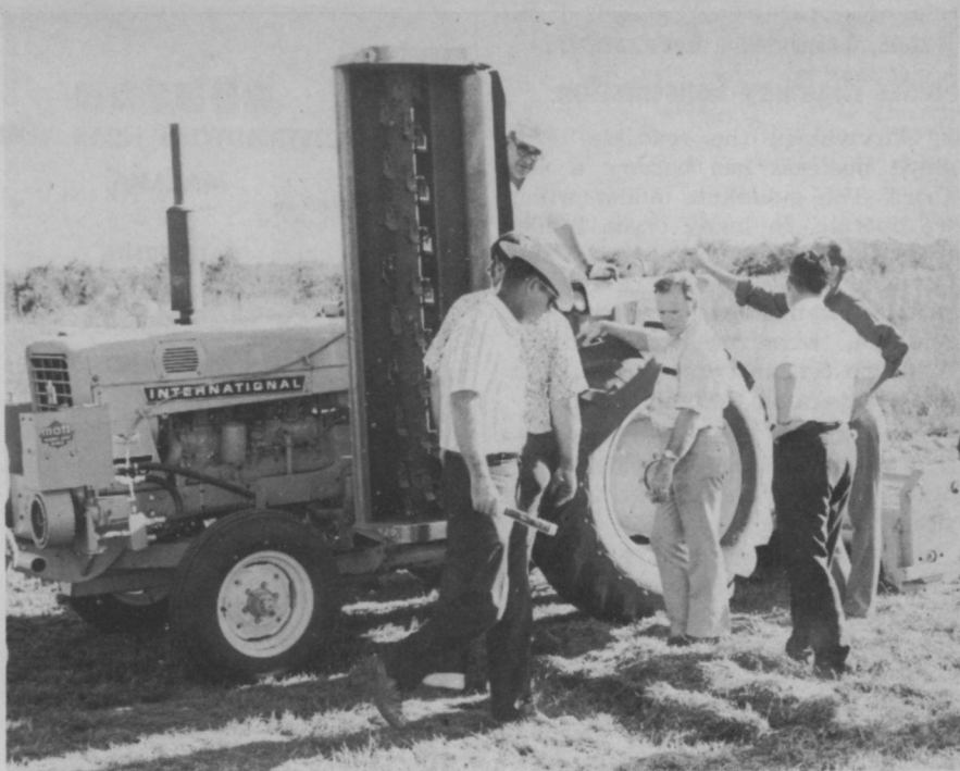
Several industry representatives inspect the cutting job done by this Mott flail mower. Complete hydraulic control makes the mower and tractor easy to operate. This unit has a wing on each side and one in the rear.
