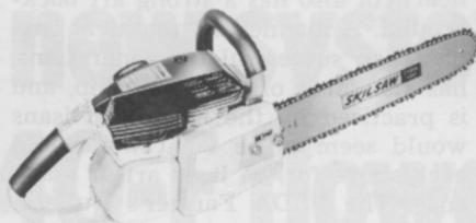
Skil saw above comes with a 4.2 cu. inch engine that's big enough to handle a 16 inch bar. Saw is well balanced.
