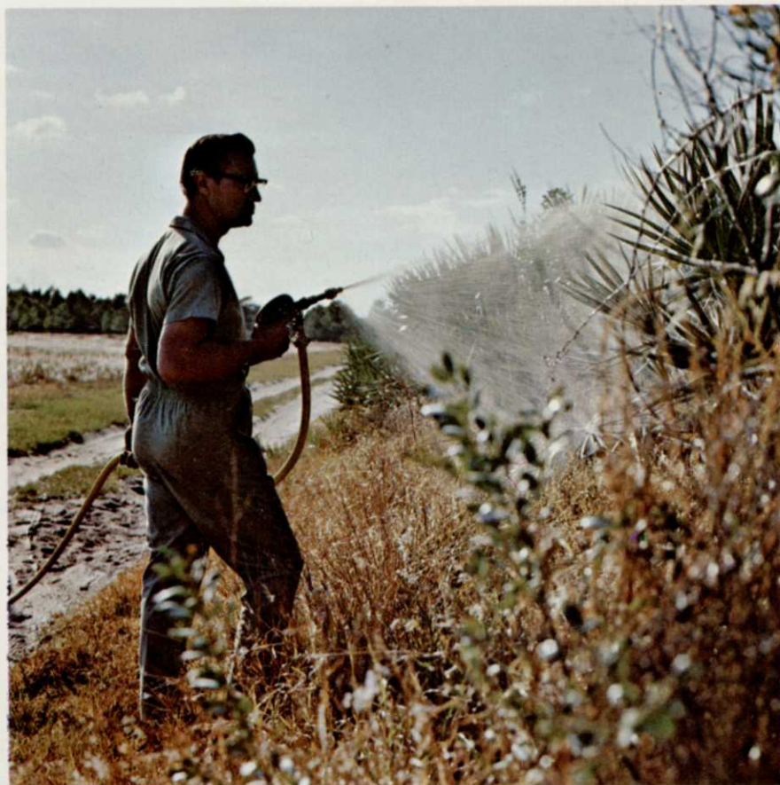
This applicator accomplishes a precision spray job with minimum drift. A variety of spray patterns are available with the Accutrol handguns.
