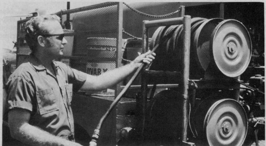
Alvin Price, above, and Dusty O'Hair, below. All Kem-Weed applicator trucks are equipped with automatic hose take-up reels and normally carry 300 feet of hose. Manifold system allows drainage of either or both truck tanks.
