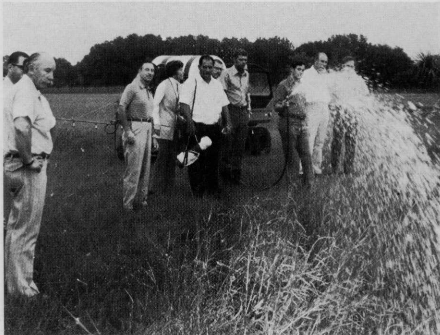
FoamSpray in action. Recently acquired from R. L. Wislon Co. by LTV Aerospace Corp., unit handles spray with reduced wind drift and helps hold chemical on foliage for longer periods.
