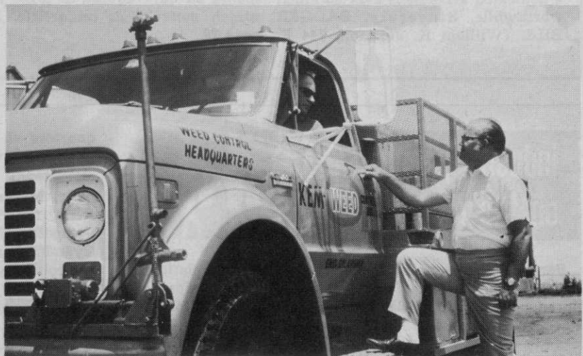
Alvin Price, above, and Dusty O'Hair, below. All Kem-Weed applicator trucks are equipped with automatic hose take-up reels and normally carry 300 feet of hose. Manifold system allows drainage of either or both truck tanks.
