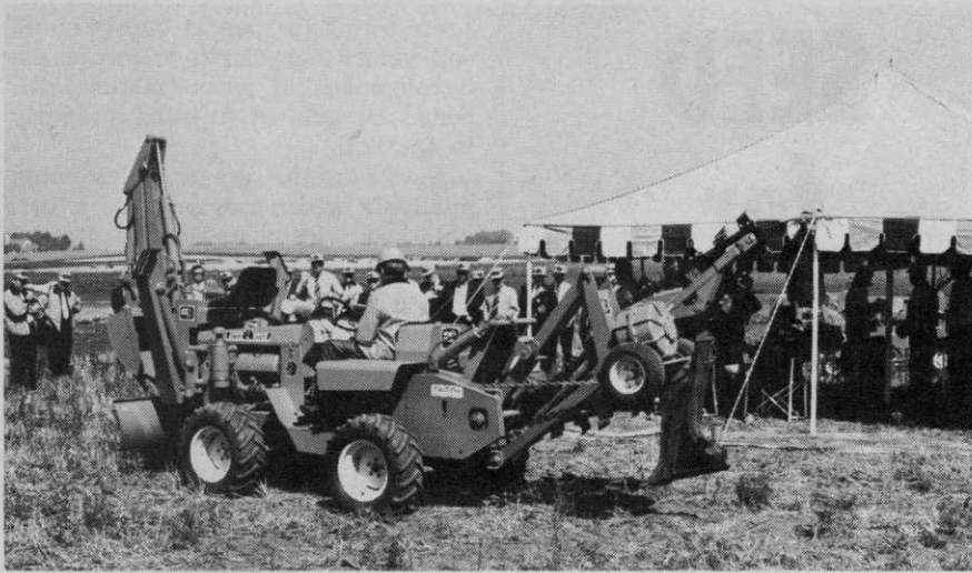
Press tent at Chicago Ditch Witch product showing. Editors see one of combo series in action. These units in various sizes do five different trenching operations, without changing or adding attachments. Combo trenches, backfills, does vibratory plowing, backhoeing, and boring.
