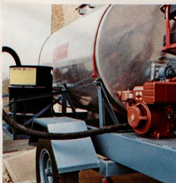
Tank is 45 \frac{1}{2} " in diameter, 6' long, with splash plate, 4 \frac{1}{2} " fill opening, large manhole for easy cleaning, sump trap to provide continued flow to pump regardless of water level. Barrel rack, shown here, is optional.
