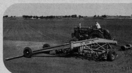
The exclusive Eversman "Hinged Frame" design permits working the field corners.
