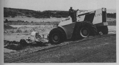
Kessen pipe-puller laying pipe. Puller works from a starter slit trench and pulls pipe through soil without trenching. On some jobs, puller can cut pipe placement time in half when compared to trenching.
