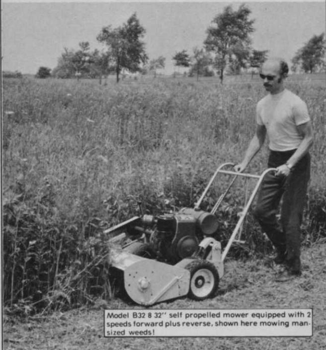
Model B32 8 32" self propelled mower equipped with 2 speeds forward plus reverse, shown here mowing man-sized weeds!
