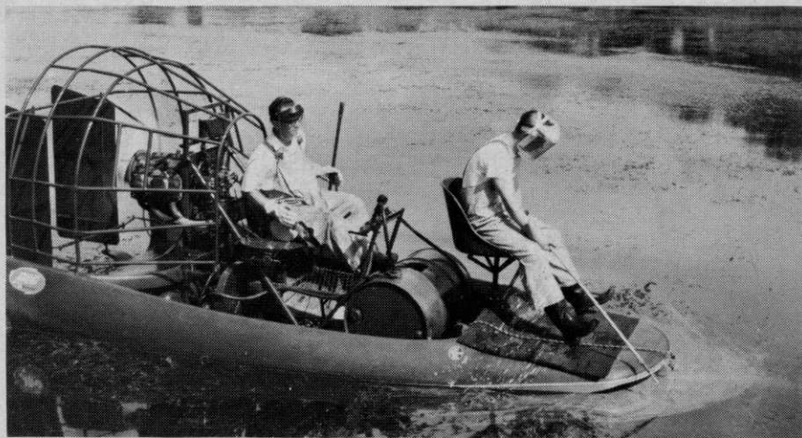
Most common method of aquatic pesticide application is airboat.
