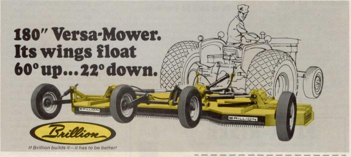
The Brillion Versa-Mower has two 5' wings that safely operate up to 60° above horizontal, or 22° below. Lets you cut a 15' swath on embankments, gulleys, rolling terrain, without scalping. Wings lift and lower hydraulically. Even fold vertical for an 88" transport width.
