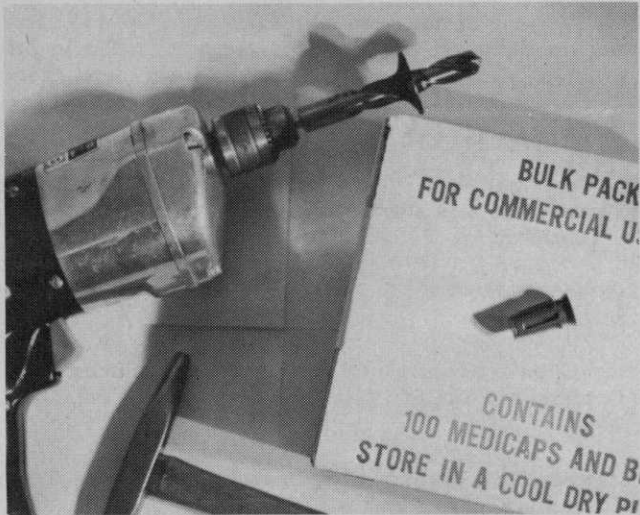
Tools for the job consist of small hammer and portable drill and bit. Bulk pack of 100 iron Medicaps will treat 20 average trees, according to Warren D. Wolfe, Creative Sales, Inc.
