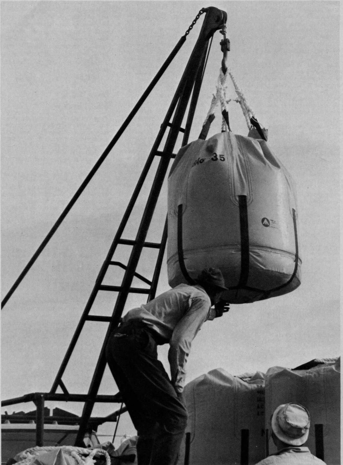
Crane handles BAG-35, a 35 cu. ft. unit, which is 40" x 51" in size. Allowable load for this size super sack is 3300 pounds.
