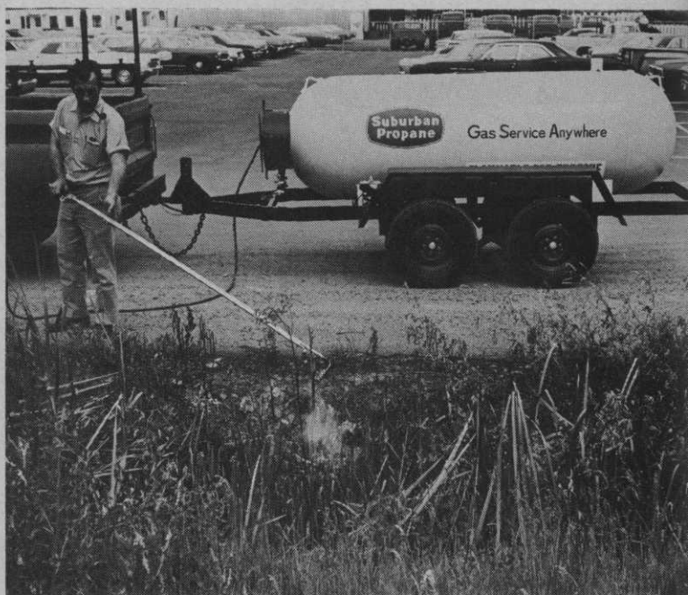
trailer-mounted tank (325 to 500 gal., water capacity) easily towed by tractor or utility vehicle. Flaming destroys weeds by exploding the cellular structure of the plant.
