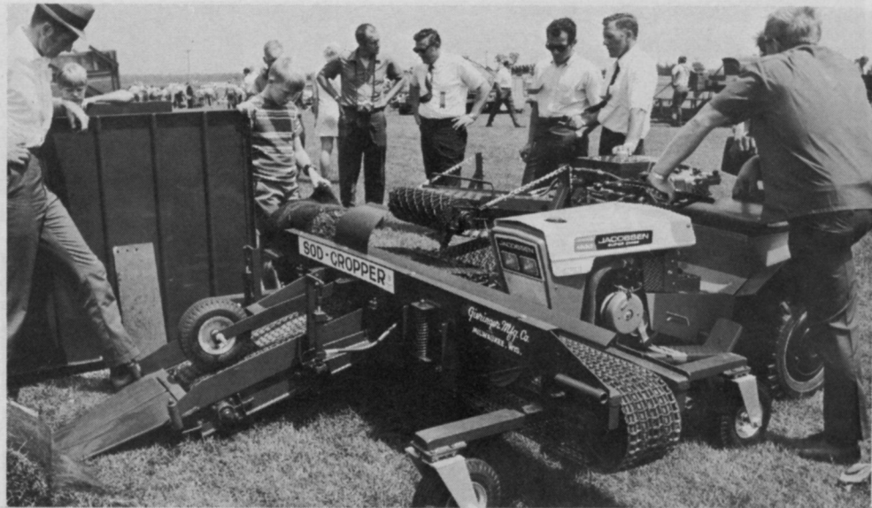
Gieringer Mfg. Co. showed its "Sod-Cropper," built around a lawn-garden size tractor.
