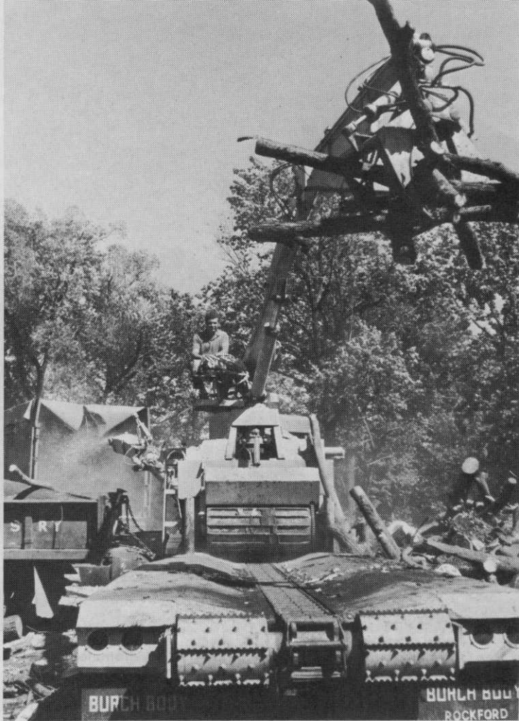
The City of Chicago has purchased a 100-ton model of the Chiparvestor, shown in action above. District Tree Foreman Jim Garvey, left, discusses its operation with Ray Toren, who's directly responsible for keeping the chipper running. A hazard, Toren says, are embedded metal objects, such as this old cable brace.
