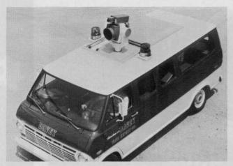
New Davey fault detection van is quickly positioned to allow automatic scanner to cover all components. An AGA Thermovision infrared camera and high resolution TV camera are mounted on a pedestal that raises the sensor gimbal through the vehicle roof and provides a weathertight inter-lock. The van also can be used for moving inspection.
