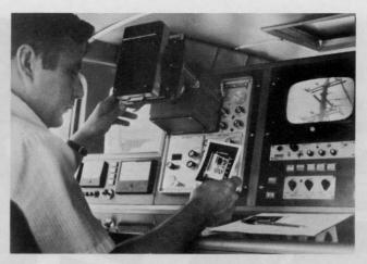
When potential trouble is detected, the operator stops the automatic scanning and measures the temperature. Variations from ambient temperature are recorded and a photograph (above) is made of the IR display to record the position of the problem component. TV view screen supplements poor resolution capabilities of the thermovision camera.
