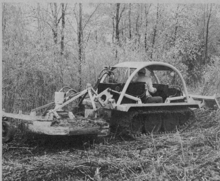
HEAVY BRUSH/GRASS TRACK-DRIVEN MOWER, Heath International, Inc., Richmond, Mich.
