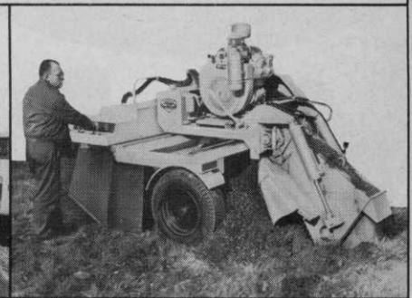
MODELS 2436 AND 2460 — Vermeer's new "reach-out" models cut wider, closer and faster. Low silhouette design. Cuts 24" deep, with 36 or 60 hp engine.
