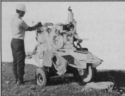
MODELS 6 AND 630 — Smallest of Vermeer's Stump Cutters. Designed for those hard-to-get-at places. Rips out stumps 6" deep. Choice of 18 or 30 hp.
