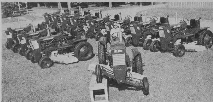
New York State Highway Department has just purchased this group of 12 slope tractor-mowers from Slope Tractor, Inc., Harper, Kan. The tractor in the foreground is simulating mowing a slope of up to 30 degrees while operator and controls remain level.
