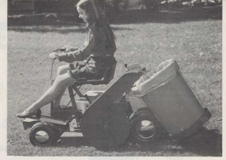
Roll out the barrel for this grass-catching mower, manufactured by Roto-Hoe Company, Newbury, Ohio. This Turf-Star Model Islander with Easy-Way Grass Catcher has a dual discharge safety deck that discharges one-half the clippings on the uncut side of the lawn, the other half into the barrel. Unit can be set to pick up all the grass or leaves. For more details, circle (719) on the reply card.
