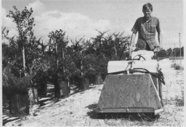
Weed-free aisles last three to four months at Cypress Creek Nursery, reports Colburn. Note the controls near the left hand. Metal bumpers at the bottom of the rig permit spraying to the edge of the cans.
