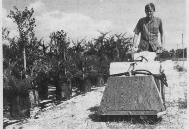
Weed-free aisles last three to four months at Cypress Creek Nursery, reports Colburn. Note the controls near the left hand. Metal bumpers at the bottom of the rig permit spraying to the edge of the cans.
