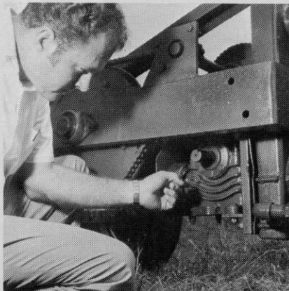
John W. Baker, sales manager, points to Turbo-Rain design features — a water turbine and gear box. The gears are driven by the turbine and pull the wheeled machine along a long steel cable.
