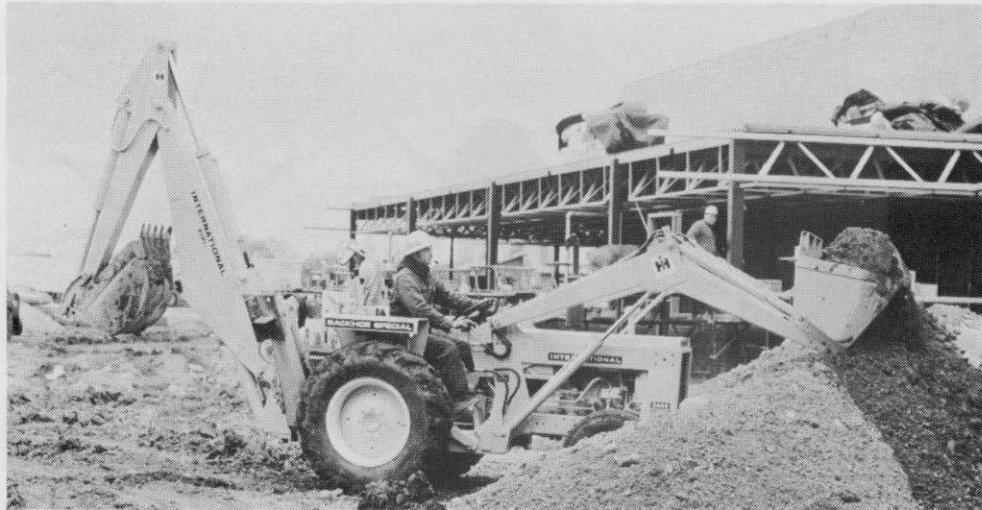
This IH 3444 Backhoe Special was among the 1970 equipment line shown at Louisville, Ky., fairgrounds. The \frac{3}{4} -yd. loader tractor with 12½ or 14½ ft. backhoe is furnished with a 73.4-inch-wide loader bucket and a 24-inch trenching bucket. It is available with a 43.5 gasoline or diesel engine, mechanical-shuttle or Hydra-Shuttle (power shift) with Torque Converter transmission.
