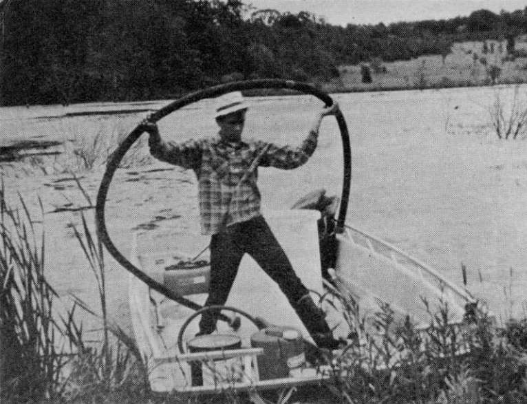
Equipment used: High-speed Homelite pump XL, 1/2-inch nozzle. Mixing (polyethylene) barrel, 2-inch intake hose with foot valve, venturi system with direct flow of chemical into water intake eliminating heavy mixing barrel, and 25 hp, 79 lb. Johnson Outboard with extended shaft. Our boat is an 18-ft. Kenner Ski Barge (fiberglass).
