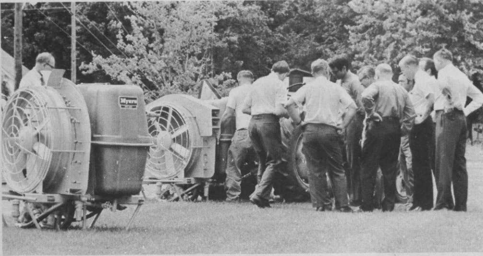
Business editors watch the hook-up of the new Myers tractor-mounted "Mitey-Mist" PTO air sprayer. It's designed for orchards, high density plantings, vineyards, turf, and field crops. Both dilute and concentrate sprays can be handled in either liquid or wettable powder form.
